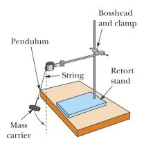
2. Using the metre rule, carefully measure the length of the pendulum from the knot at its top to the base of the mass carrier. Enter this length in table 13.1A.
